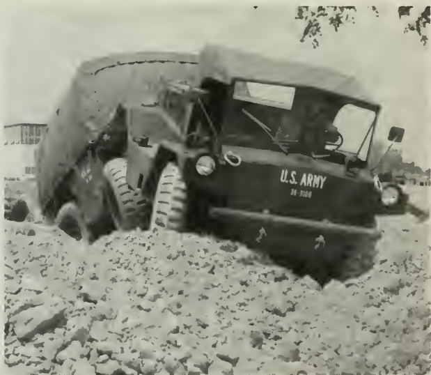
ARMY is testing XM 561 jointed cargo carrier, which goes equally well in the water (left) or over roughest terrain.
